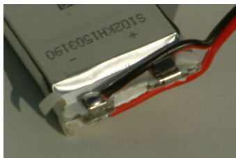
A 2-cell LiPo battery minus its heat shrink sleeve, showing the cell's connecting tags.
