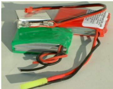
A collection of LiPo batteries. The delicate silver metalised Mylar skin of the cells may easily be seen. Heat shrink sleeve is used to hold the cells securely and to cover the cell's connecting tags. Note also the use of a protective sleeve on the positive lead of the red battery, which is fitted with 2mm 'Gold' connectors
