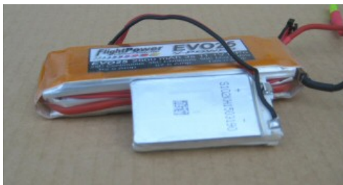
Old and new. The small early battery was rated at just 3C. Several years of development have provided modellers with some remarkable improvements. Modern high performance LiPo batteries are now able to deliver a sustained discharge current of 25C or even 30C.
